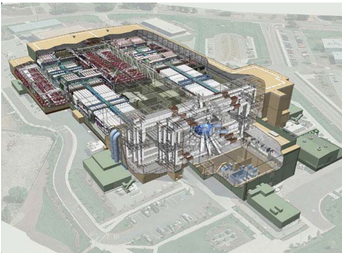
Fig. 9 The National Ignition Facility (NIF) at Lawrence Livermore National Laboratory (LLNL), the world's largest laser. The 1.8 MJ of ultraviolet light (351 nm wavelength from frequency-tripled neodymium:glass laser light) is generated with precision pulse shaping in the left and right laser bays and routed to the spherical target chamber in the lower center of the picture. The scale of the facility is illustrated by the fact that three American football fields could fit inside the NIF building. (Courtesy of Lawrence Livermore National Laboratory)
