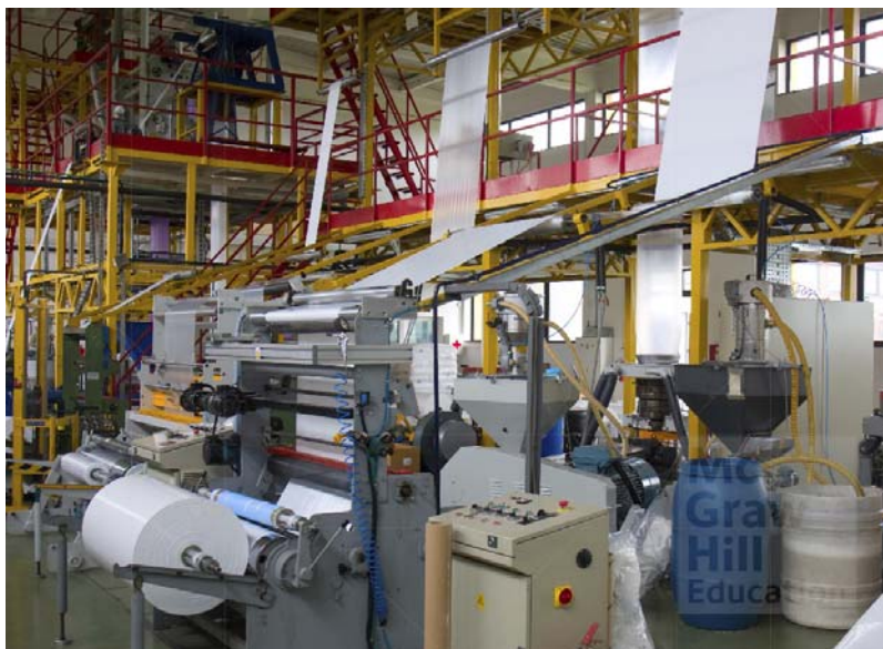
Fig. 1 Polymer extrusion process for making plastic bags. (Credit: firemanYU/Getty Images)
